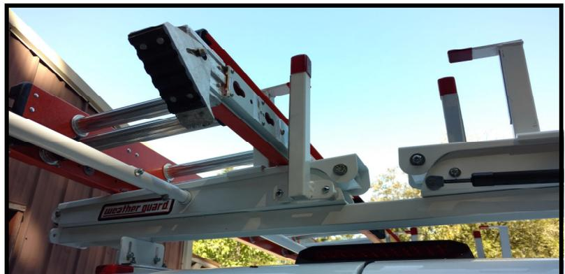
Streamlined at only 1/2" depth to minimize interference with racks
